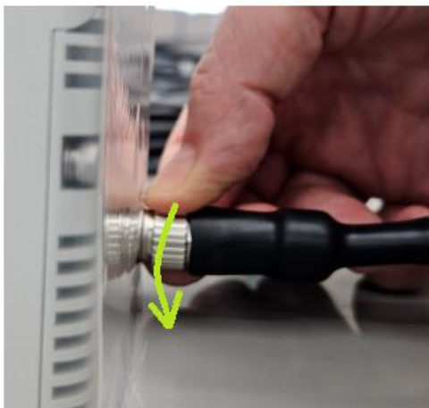
Figure 5: Power and data cable withdrawal instructions
